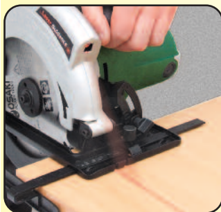
Laser guidance for precision cutting.
