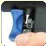
Forward/Reverse lever action.
