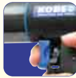
Two speed trigger for slow or fast action.
