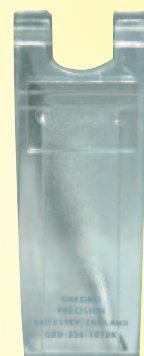
Lens for Portable Refractometer
